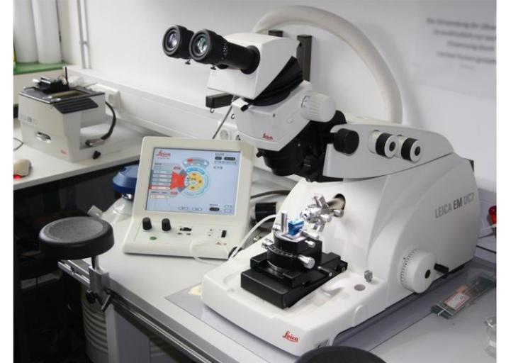
Leica Ultracut EM UC7 ultramicrotome
